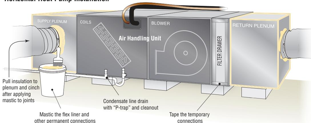
Whether a heat pump or a fuel-fired furnace, foundation-located HVAC systems need proper attention to details such as: adequate drainage for water condensation from the evaporator coils, mastic sealant on permanent joints of the air handler unit and ductwork, taped seams of temporary enclosures such as the filter drawer and attention to regular maintenance needs.
